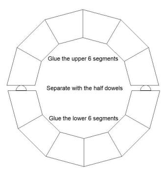
3. When you clamp this way all segments are forced together with no gaps, all the error is transferred to the ends of the 6 segment sections. Once the glue dries you remove the clamp and
