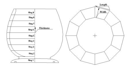
3. There are 10 rings so you will need 10 blanks. These blanks must be straight and flat. If you use a blank that has a bow or twist it can adversely affect the angle you cut and that will cause a gap when you glue up the ring. So use care when you select and cut the blanks. The
