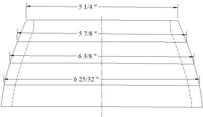
carefully fit the lid to the vessel. You do not want a snug fit, but at the same time you don't want a loose fit either.
