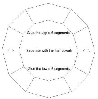
3. When you clamp this way all segments are forced together with no gaps, all the error is transferred to the ends of the 6 segment sections. Once the glue dries you remove the clamp and
