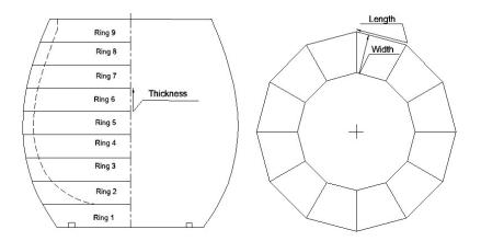
3. There are 10 rings so you will need 10 blanks. These blanks must be straight and flat. If you use a blank that has a bow or twist it can adversely affect the angle you cut and that will cause a gap when you glue up the ring. So use care when you select and cut the blanks. The
