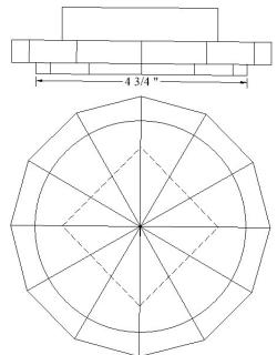
6, Turn a tenon on the bottom of the ring to a diameter of 4 3/4" and 1/4" deep.
