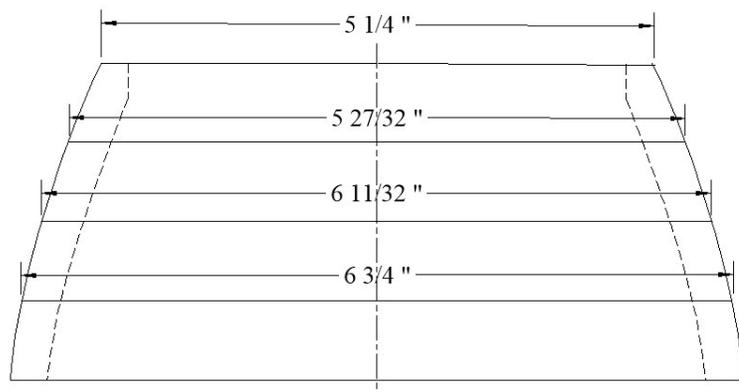
12. Following the same steps as before, glue the other 4 rings to the vessel and turn the outside to the dimensions show here.
