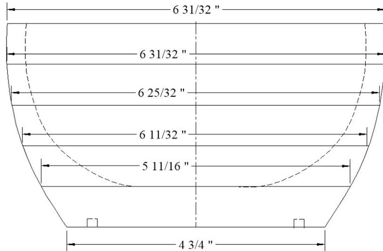
11. Remove the jig from ring 2 and apply ring 3 to it. Glue up ring 3 in the same way you did ring 2. Repeat these steps until you have five rings glued up. Allow them to dry overnight and you are ready to start turning the vessel. The illustration to the right shows all the dimensions you will need to turn this portion to the correct shape.
