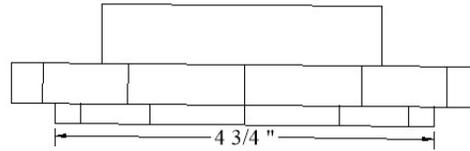
5. Start with a 2 1/2" square sacrificial. You will attach ring 10 to the sacrificial with double sided tape (Carpet tape). Align the corners of the sacrificial with the joints of every third segment. See the drawing to the right. Once the sacrificial is secured to ring 10 place the assembly in a 4 jaw chuck.
