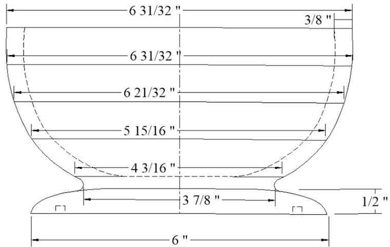
11. Remove the jig from ring 2 and apply ring 3 to it. Glue up ring 3 in the same way you did ring 2. Repeat these steps until you have five rings glued up. Allow them to dry overnight and you are ready to start turning the vessel. The illustration to the right shows all the dimensions you will need to turn this portion to the correct shape.
