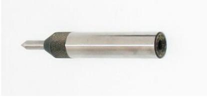
The tap guide is placed in the same drill chuck you just used to drill the hole. It has a spring loaded center point that goes in the hole in the end of the tap. The setup looks like this.
