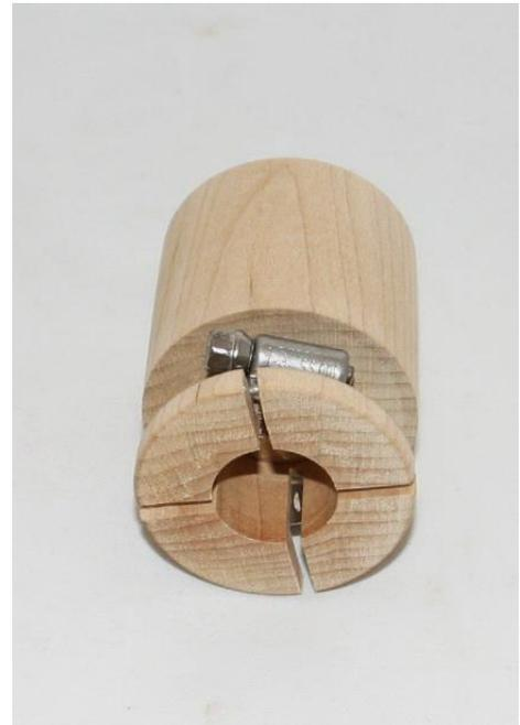
This is built very much like the tail stock jam chucks except that you drill and tap the end to match your head stock spindle. The collet end is sized to fit a specific diameter and then "split" with a table saw and uses a hose clamp for tension.
